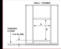
The rough framing dimensions shown represent the distance from stud to stud only and do not take into consideration the addition of drywall. Please refer to installation instructions for complete specifications and drawings when installing this product. Go to heatilator.com to download.
